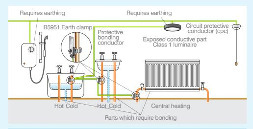
Earthing Conductor A protective conductor connecting the main earthing terminal of an installation to an earth electrode or other means of earthing.
